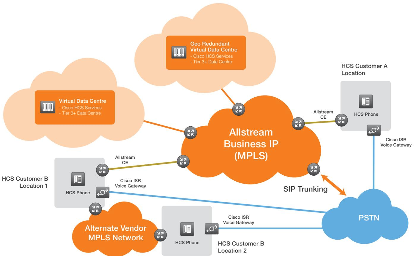
The diagram illustrates the architecture of Allstream HCS. Customer A operates one business location while Customer B operates two sites connected with an MPLS network from an alternate vendor. Allstream includes the cost of the connectivity from the Allstream HCS hosting location to the Allstream SIP trunking network as part of the per user price (highlighted in orange). MPLS connectivity from the customer site to the Allstream HCS hosting location is engineered and priced separately.
